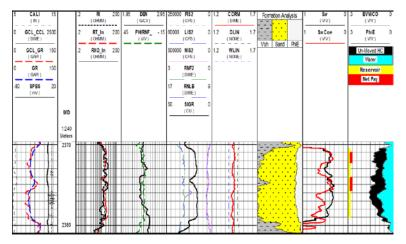
7-5/8 in hole with 5-1/2 in casing. The lithology corresponds to a sequence of sandstone and shale. The formation water salinity is approximately 5 Kppm.
